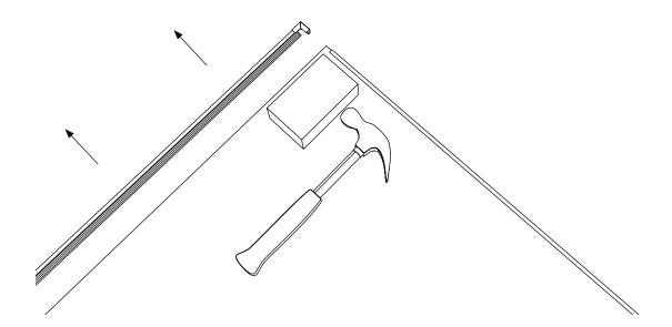
2. Remove the frame, including the pen shelf, from the whiteboard. Separate the aluminum and plastic corners.
